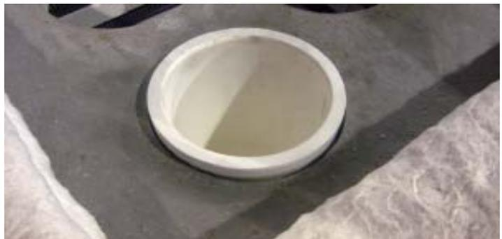
Your furnace has been fired at our factory to cure the refractory and test the electrical circuitry. We fired the unit for a 24 -36 hour period to "set" the castable, which optimizes their strength. The first firing at customer location should be done with attention and care as it will significantly effect the life of the castings.
